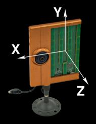
Amplitude: signal strength X: R x sin( $\theta$ ) Y: R x cos( $\theta$ ) x sin( $\Phi$ ) Z: R x cos( $\theta$ ) x cos( $\Phi$ )
