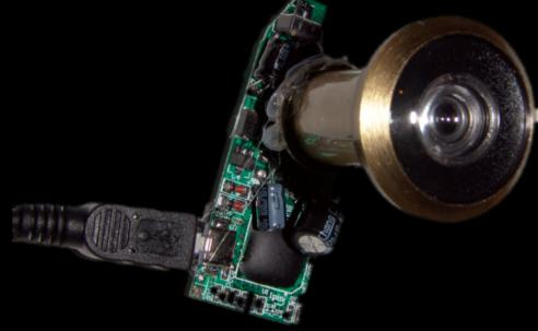
Cameras: 3 webcam Control: USB tether Purpose: 360° augmented reality to guide firefighters in burning buildings
