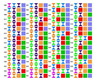
Wiring the cluster with the GA design took no more than a few minutes per PC, including the time to neatly route the wires between the PC and the switches. In fact, we re-ran the GA to optimize for the communication patterns of the DNSTool CFD (Computational Fluid Dynamics) code [4] and physically re-wired the entire system in less than a few hours. The new design is:
