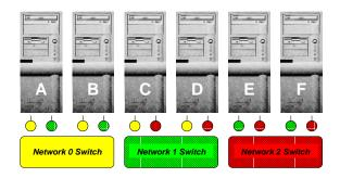
Thus, A and B are both connected to switches 0 and 1, C and D to switches 0 and 2, and E and F to switches 1 and 2. For A to send to C, it uses switch 0. For A to send to B, it can use either switch 0, switch 1, or both.
