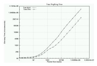
In contrast, the FNN both has lower latency (due to all paths passing through only a single switch) and the One and Multi cases achieve virtually identical performance:
