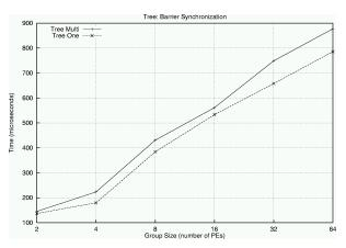
Aside from being generally faster than the tree, the FNN should not suffer a significant penalty for the Multi case. As the following figure shows, there is indeed no penalty for the Multi case; in fact, the Multi case is even slightly faster for groups of size 16 or 32 PCs:
