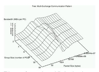
This tree performance is especially daunting when one realizes its implications on "channel bonding." Even if we were to duplicate the entire switch tree for 5-way channel bonding, and have the channel bonding be 100% efficient, all of that hardware would yield about 5 times 1.36MB/s, or 6.8MB/s! Worse yet, that is a peak number achieved only for a specific group size and message length... the average performance is even poorer.
